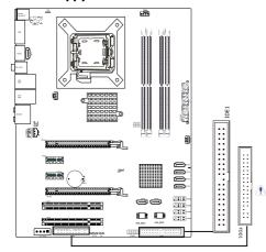
Each of the IDE port connects up to two IDE drives at Ultra ATA/100 mode by one 40-pin, 80-conductor, and 3-connector Ultra ATA/66 ribbon cables.
